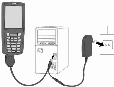
Figure 2-11 Communication through Cable
